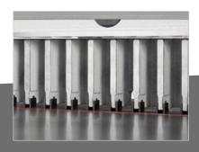
Backgauge rakes with plastic gliders treat the table surface with care
