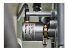
Direct measurement via rotary transducer flanged to the spindle
