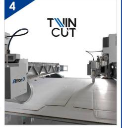
Cutting area up to 3200x2200 mm with suction surface made up of 24/32 sectors for the perfect adherence of the materials, even the most critical ones.
