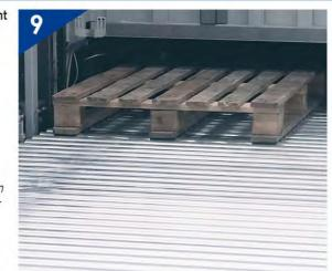
The material handling can be equipped with roller conveyors or Acetal mats, for the unloading functionality and even partial handling, up to the single sheet.
