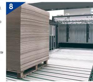
Automatic management of the pallets recovery from the loading area to the unloading area. Original solution, patented by Elitron
